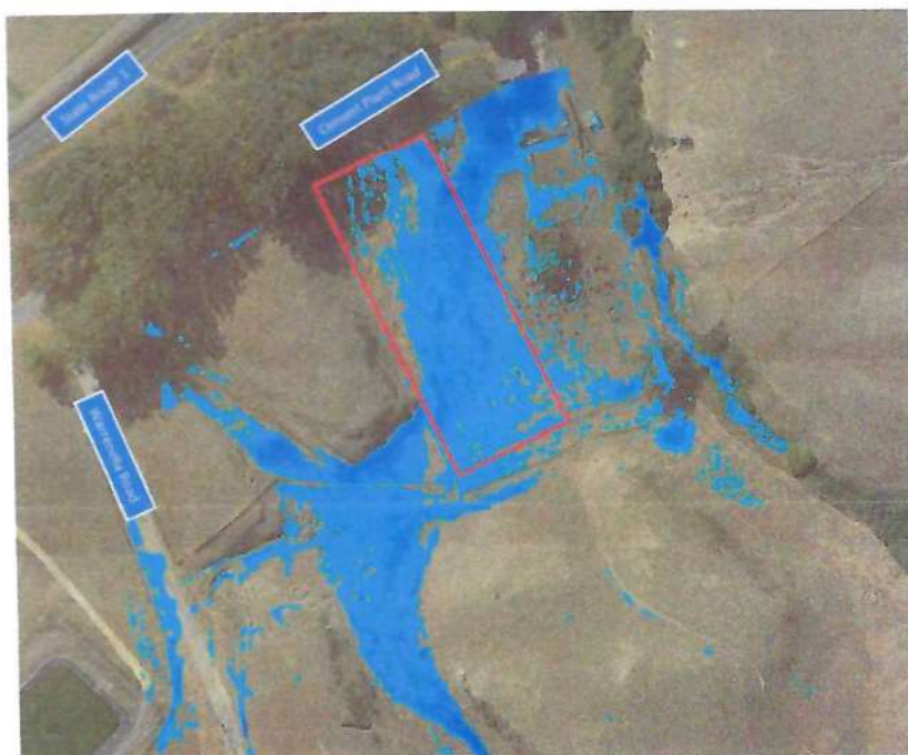
Fig 2. Two-dimensional model for a 9.5-inch storm over a 24-hour period. EA page 23
